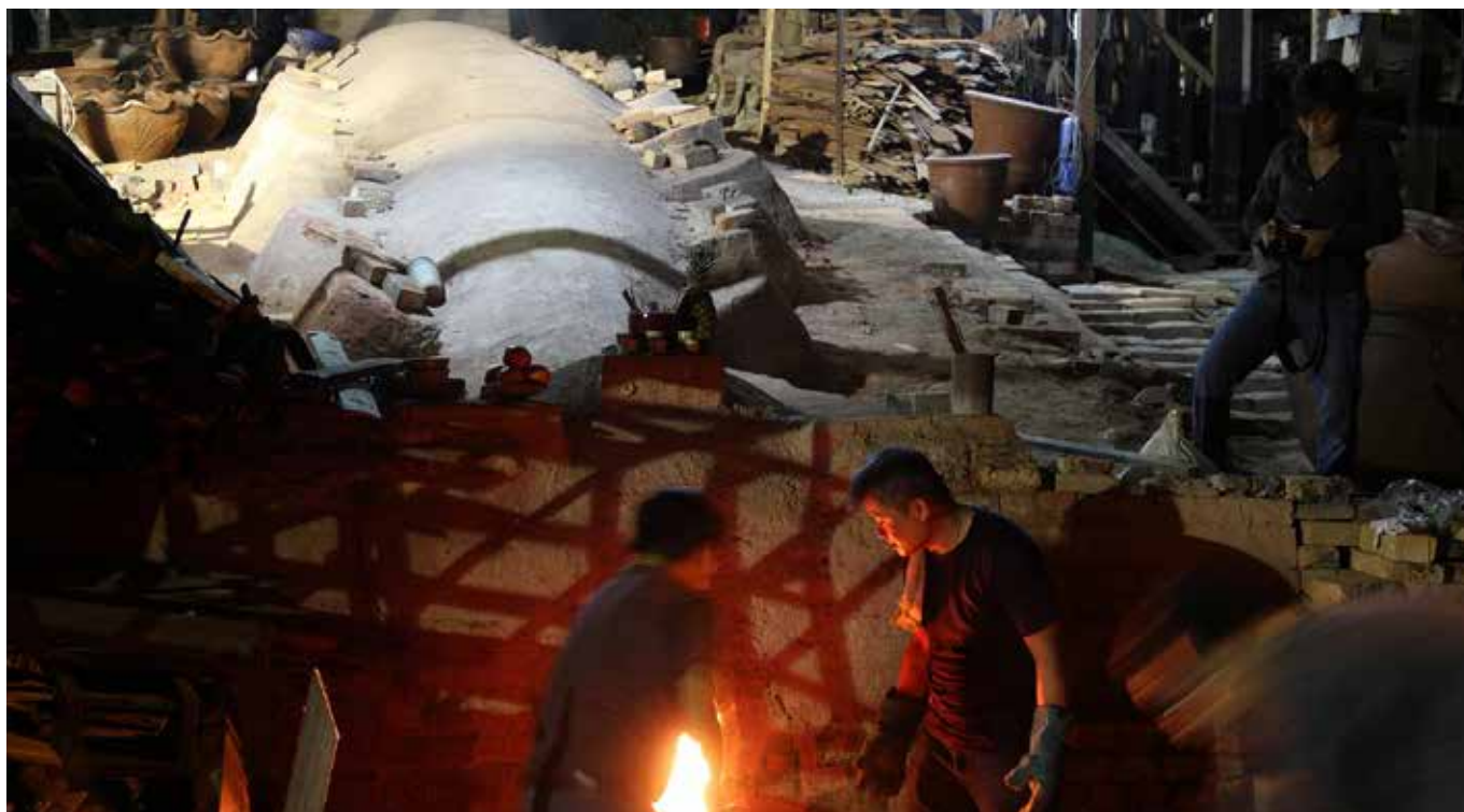
Wood being fed manually into the firing box. An altar to the kiln can be seen on top.
